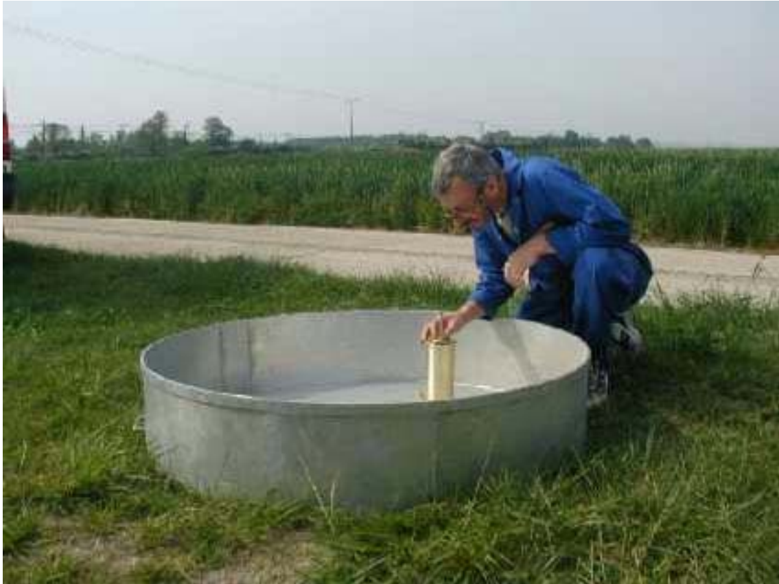
Class "A" Evaporation Pan (ref : FM9002) with Hook Gauge (ref : FM9000) and Still Well (ref:9001 - Order separately)
